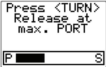
Release the button when the rudder reaches the port hard over position.
