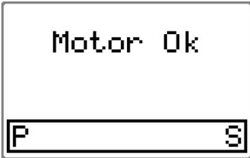
The **Rudder test** is verified by the display showing 'Motor OK' or 'Failed'. If 'Failed' is given, check for correct electrical connection.
