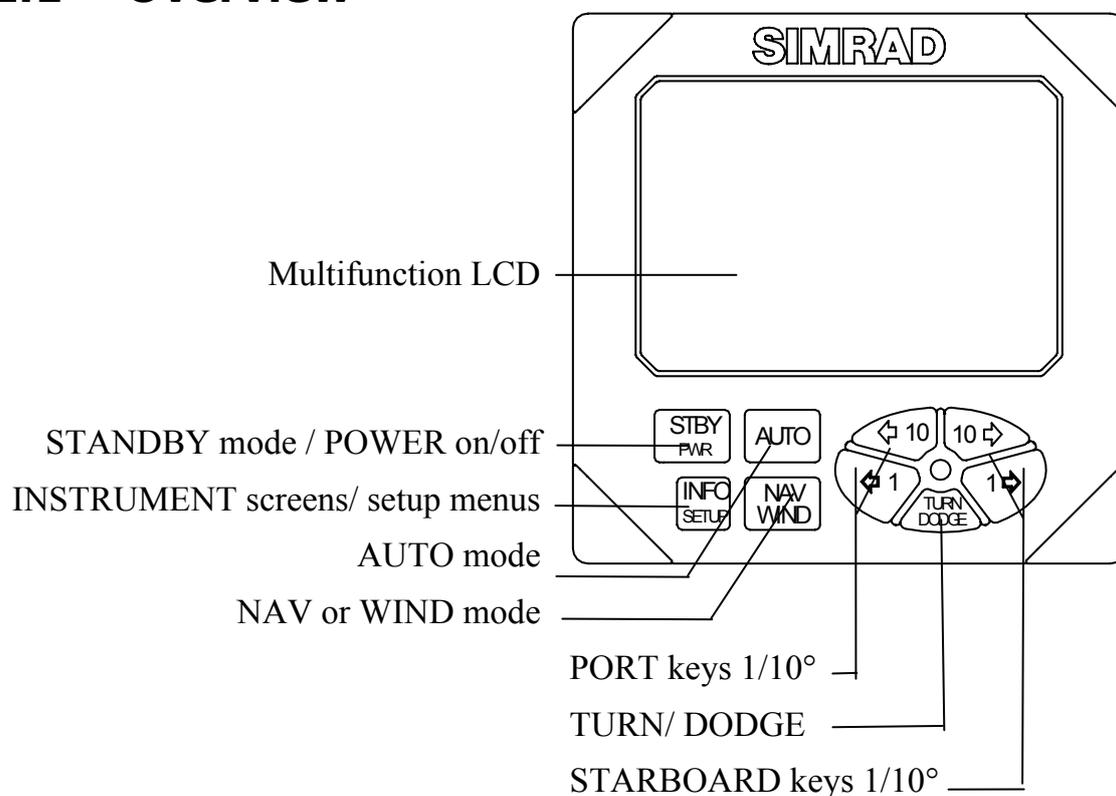
The control unit shown above can operate as a stand alone unit in an autopilot system or combined in a multistation system. In a multistation system the command can easily be transferred from one unit to another. AP16 units not in control will display the ☒ icon.
