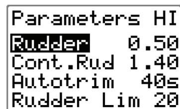
A boats steering parameters found by the Automatic tuning can be looked at and if needed changed under this menu item. The steering parameters can also be set manually instead of
