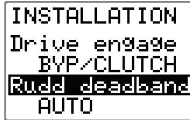
The rudder deadband function is adaptive and is continuously operative. It prevents the rudder from hunting and the adaptive function optimizes the deadband to the speed of the boat and the pressure on the rudder.
