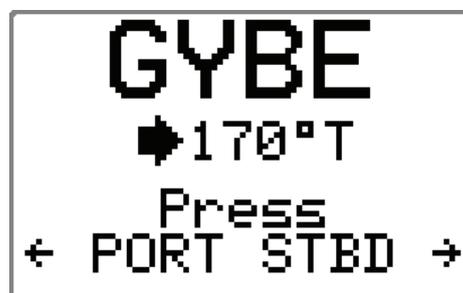
When a gybe is initiated, the wind angle will first be set to 170°T on the same side as the current wind angle. The main sail should now be hauled. With the main sail safely hauled, the wind side may be changed. This is done by pressing either **PORT** or **STBD** buttons depending on the way the boat should continue to turn. The new set wind angle will then become the same as the wind angle set before the gybe operation started.
