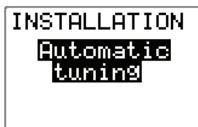
Activate the *Automatic tuning*, by pressing the **STBD 10** button. The display will flash “Automatic tuning”.
