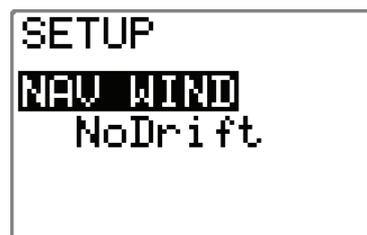
Select NoDrift in the Setup menu when in **STANDBY** or **AUTO** mode. Press the **NAV WIND** button to enter NoDrift mode. The **NAV WIND** key is now programmed to always activate the NoDrift mode. If you want the key to activate NAV mode, enter the User Setup menu and select NAV.
