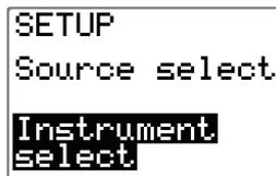
Select the instrument page(s) to be available under the **INFO/SETUP** button. Step through the list of instrument pages by using the **PORT 1** or **STBD 1** button. Select the wanted pages by filling the squares with the **PORT 10** or **STBD 10** button.
