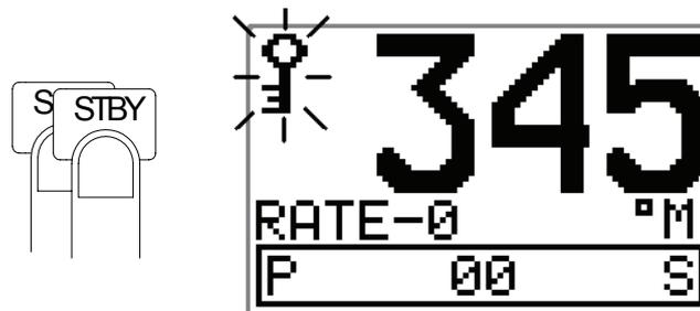
The display on the active control unit will first show a
