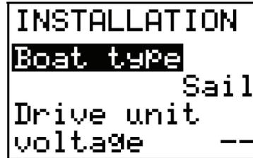
Actual boat type is selected by pressing the **STBD 10** or **PORT 10** buttons. The options are: Planing, Displacement, Sail and Outboard.
