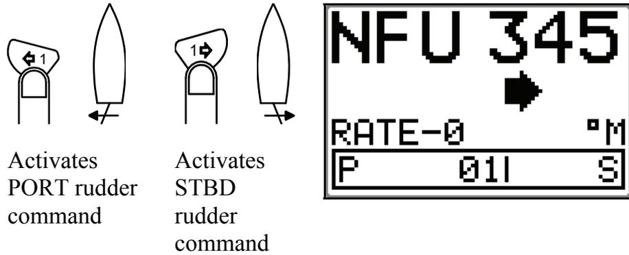
**Note !** *When a NFU steering lever or remote control is operated, other control units become “Inactive”.*
