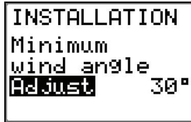
The 'Minimum wind angle' is the minimum apparent wind angle that will keep the sails well shaped and give an acceptable thrust. This parameter will vary from boat to boat.
