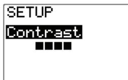
The contrast of the display may be adjusted to 10 levels (10 = highest contrast). The setting is stored when the system is turned off.
