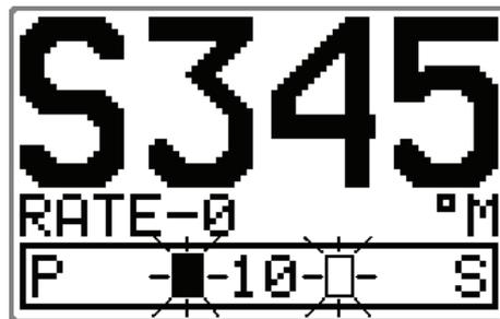
After turn on the rudder angle display will alternate between 10 degrees port and starboard to indicate that the "rudder" zero point need be set.
