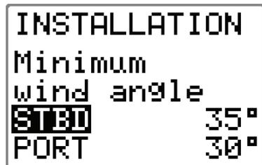
If 'Wind setup' is set to RACING, you can set different minimum wind angles for port and starboard. The difference between port and starboard wind angles will be taken into account when calculating the Estimated Time to Turn (ETT) and Distance To Turn (DTT).
