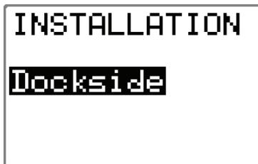
Press and hold the **INFO/SETUP** button to enter the Installation setup menu. Select "Dockside" and press the **STBD 10** button to open the "Dockside" menu. This will automatically configure the autopilot for Virtual Feedback, and the alternating feedback alarm will disappear from the display.
