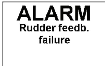
At first time turn on the autopilot will after approx. 5 seconds sound and display a feedback failure alarm. Press the **STBY** button to silence the alarm and follow the instructions in the display to initiate the Setup as described on page 83
