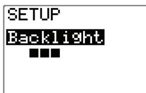
The backlight of the display and buttons may be adjusted to 10 levels (10 = brightest). The setting is stored when the system is turned off. Adjustment is local to the control unit you adjust or synchronized with other units in the Simrad Group (page 116).
