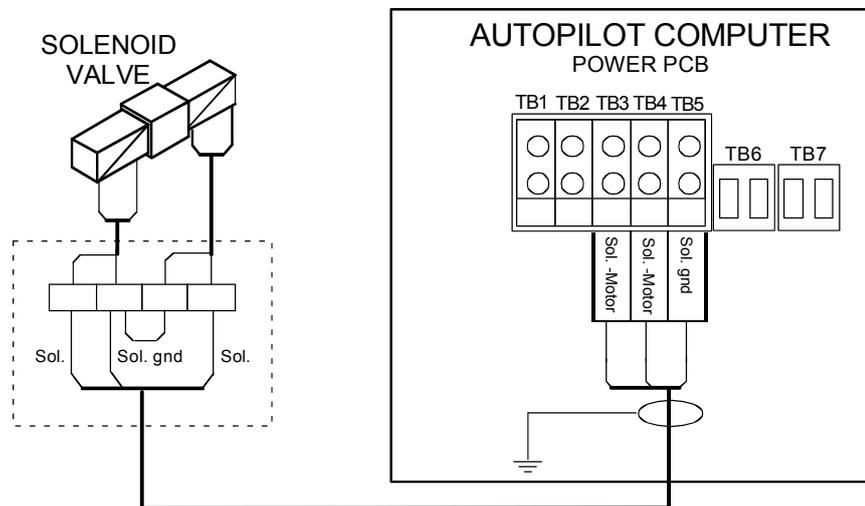
Figure 3-7 Connecting a solenoid valve
