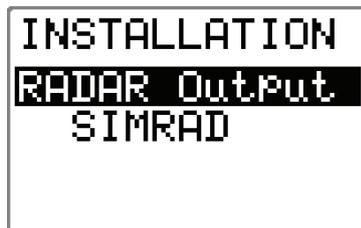
Use the **PORT 10** or **STBD 10** buttons to select the connected type of radar.
