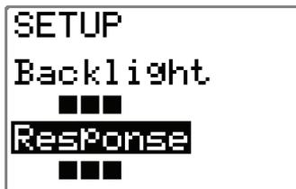
The Response control allows you to make this fine tuning. It can be set to seven levels. Level 3 (default) has the values of *Rudder* and *Counter Rudder* parameters set by the Autotune function. If no Autotune is made (not recommended) the level 3 values are the factory default values.
