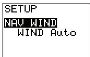
If 'NAV WIND' is set to 'WIND Auto', wind steering will be enabled. Pressing the **NAV WIND** button will then initiate the WIND-mode. The autopilot will automatically select between apparent and true wind steering.
