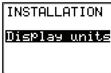
Select *Display units* by pressing **STBD 1** button and confirm by pressing the **STBY 10** button. The setup is local to each control unit.
