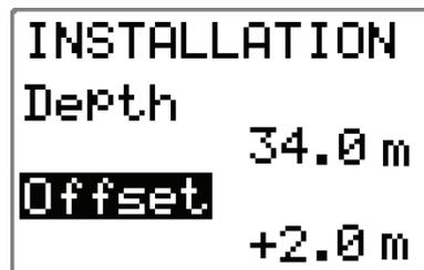
When the depth offset is set to zero, the indicated depth is from the transducer to the bottom.
