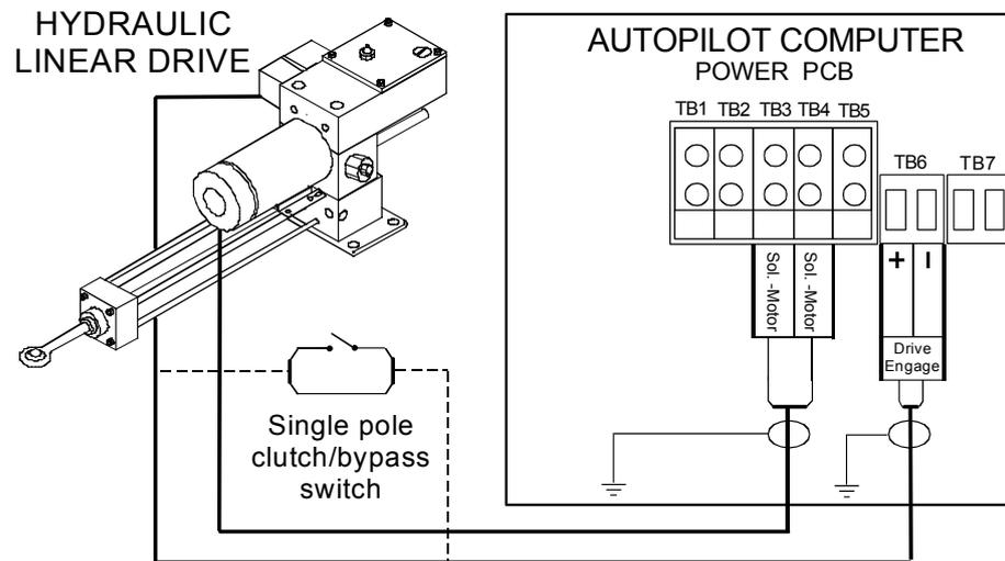
Figure 3-6 Connecting a hydraulic linear drive
