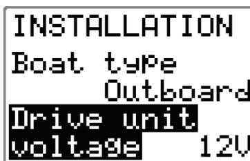
When the autopilot is configured for Virtual Feedback the *Boat type* is automatically set to *Outboard*.
