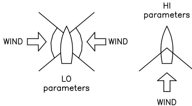
The transition between HI and LO parameters and vice versa will have a different characteristics with regards to the wind angle compared with the transition controlled by the speed of the boat.
