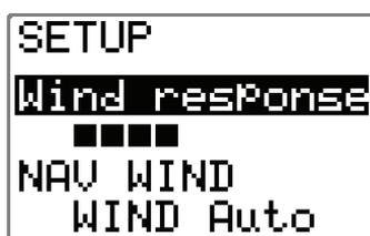
The User setup menu for WIND mode is the same as for NAV mode. In addition you have:
