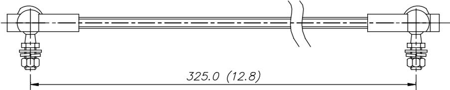
Figure 8-6 Transmission link - Dimensions
