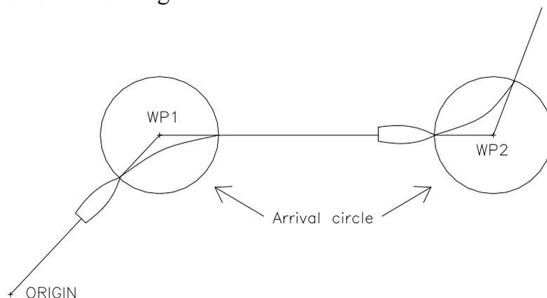
The figure below may be used to select the appropriate waypoint circle on the GPS/chartplotter.
