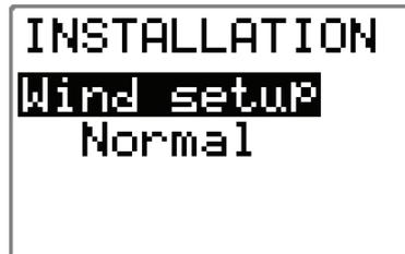
Wind setup has two levels: NORMAL and RACING. The RACING level will give access to more wind setup items to achieve optimal performance when sailing. Additional setup items also become available in the User setup menu.
