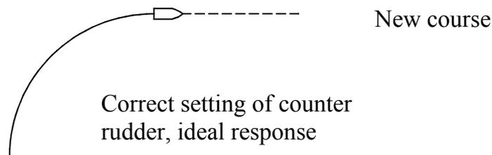
**Autotrim** standard value is 40 sec. which should work well on most boats.
