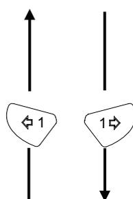
Use **PORT 1** and **STBD 1** buttons to step through parameters
