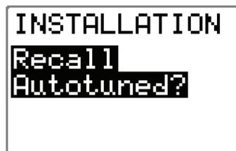
To recall the parameter values that were achieved during the *Automatic tuning* procedure, press the **STBD 10** button. When parameter values are recalled, *Confirmed* is displayed.
