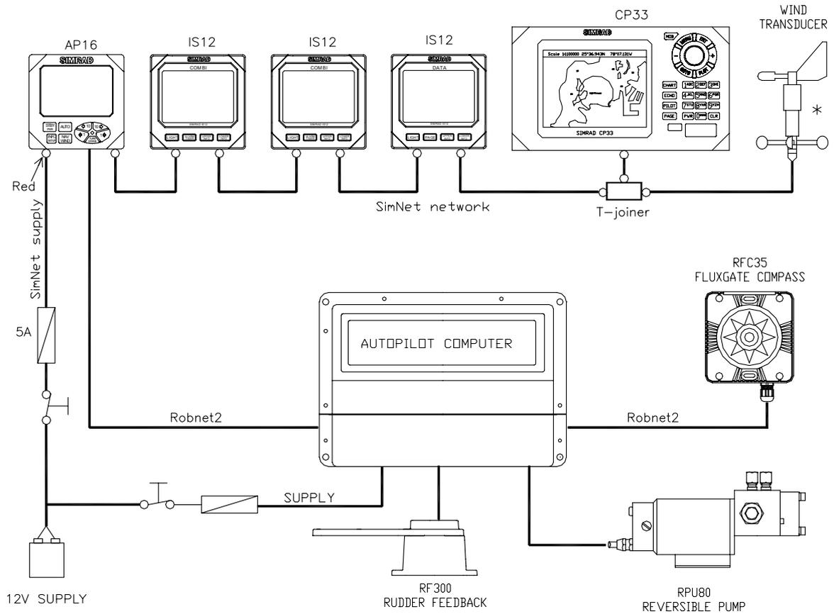
Figure 3-19 Robnet2 and SimNet network
