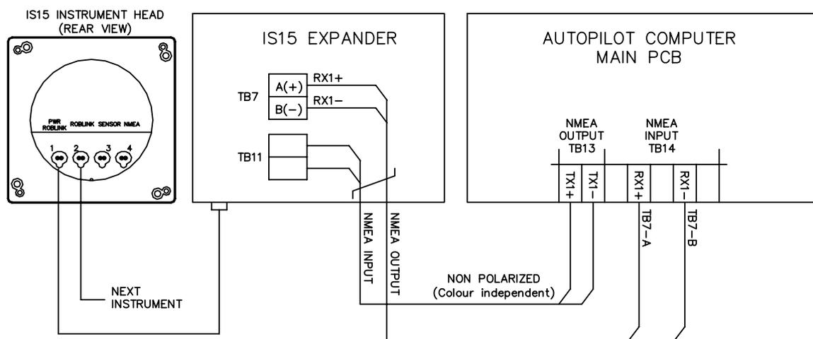
Figure 3-26 IS15 Expander / Autopilot computer connection
