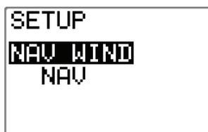
This setup will configure the active mode under the **NAV WIND** button. The following alternatives are available:
