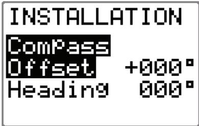
Select the amount of correction by pressing the **STBD 10** or **PORT 10** buttons to offset the heading to agree with the known, accurate heading. The *Offset* value can be either positive or negative.
