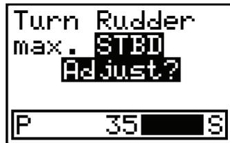
The value on the display is the angle read by the rudder feedback unit before any adjustment is made. If the actual rudder angle is different from that of the display, correct the reading by pressing the **STBD 10** button to increase the value or the **PORT 10** button to decrease the value (see note).
