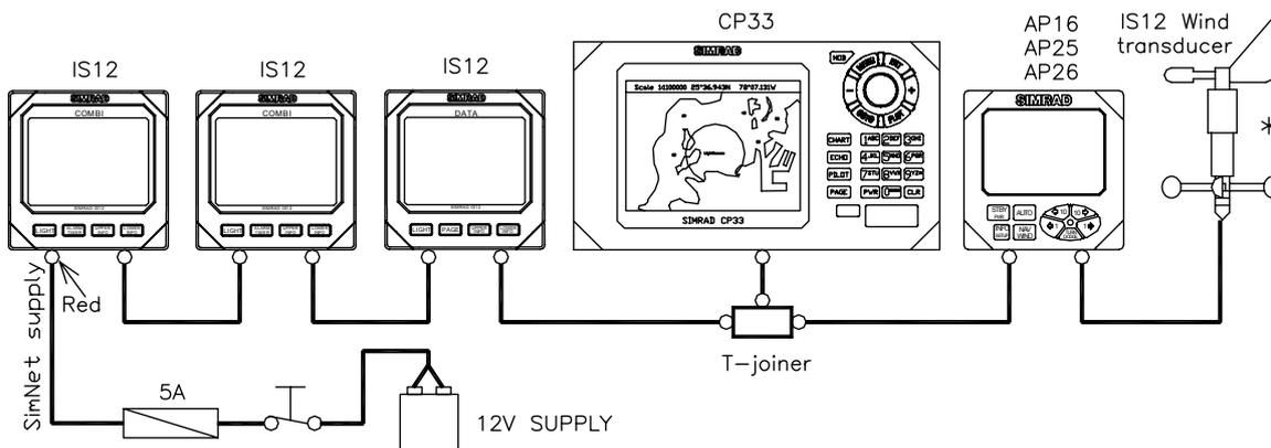
Figure 3-17 SimNet network, small system with Wind transducer
