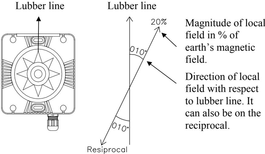
**Note !** *In certain areas and at high latitudes the local magnetic interference becomes more significant and heading errors exceeding  $\pm 3^\circ$  may have to be accepted.*
