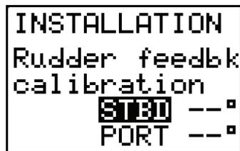
Confirm Rudder feedback calibration to STBD by pressing the **STBD 10** button. You will read dotted lines only the first time you enter this screen.
