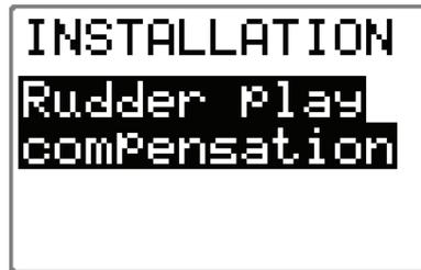
This adjustment must be made when steering in dead calm sea. Confirm by pressing the **STBD 10** button.
