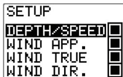
Available instrument pages are: Depth/Speed, Wind App., Wind True, Wind Dir., Track data, Nav data, Position and Temperature.
