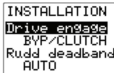
This determines the use of the autopilot computer drive engage port (Bypass/clutch terminals). The port voltage is the same as the selected drive unit voltage. Drive engage has the following settings:
