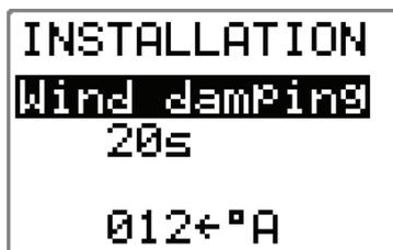
Damping of the apparent wind angle is made by the Advanced Wind Filter (AWF) in the Autopilot Computer. The inputs to the AWF are heading, boat speed, apparent wind angle and wind speed. Verify that these inputs are available in User Setup/Source Select (page 42).
