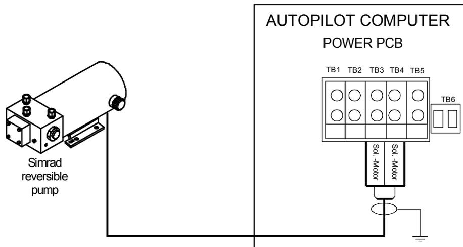
*Figure 3-5 Connecting a reversible pump*
