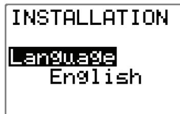
The Installation Menu is presented on the autopilot display by pressing and holding the **INFO/SETUP** button for 5 seconds.
