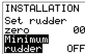
Turn the minimum rudder on by pressing the **STBD 10** button.
