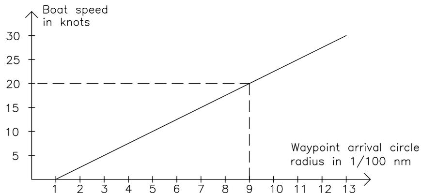
Example: With the speed of 20 knots you should use a waypoint circle with radius 0.09 nm.
