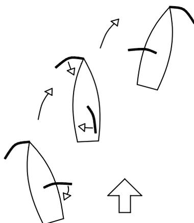
The rate of turn when changing wind side in a gybe will be the highest possible, determined by the performance of the drive unit.
