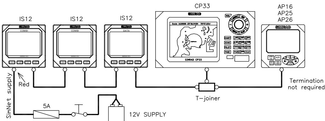
Figure 3-16 SimNet network, small system
